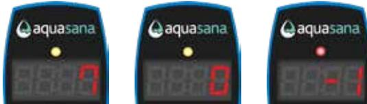
At any point during this sequence, the audible chirp or alarm can be deferred for seven days by holding the controller button down for a period of five seconds. The number of deferrals used will be displayed as below. Once the deferral expires, the alarm will sound once again. The deferral can be repeated up to three times. PLEASE NOTE: At any point after lamp expiration, the water may be unsafe for consumption and should not be consumed without another form of disinfection.
