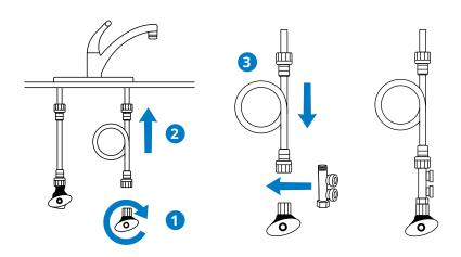
Connect 3/8" tubing to the bottom port of the Dual Port Adapter. Run the opposite end of the tubing to the inlet side of the System Head (marked "IN"), cut to length, and push tubing into the inlet until it stops.
