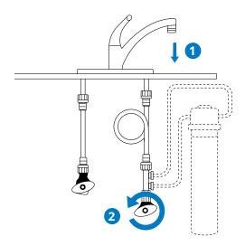
**9** Leave water running to flush cartridge for 15 minutes or until water is clear of carbon fines. While the system is flushing, check for leaks. Once the system is flushed, turn off kitchen faucet.
