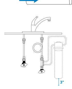
Three (3) inches of clearance from the base of the cartridge is needed for easy cartridge replacement.
