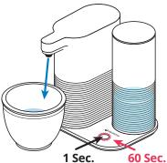
6. Once the flush is complete, light blinks blue for 5 seconds, then illuminate solid blue for 5 seconds.
