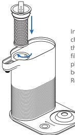
Insert the filter with the attached filter chamber cap onto the chamber so that the grooves of the cap line up. Twist the filter chamber cap to the right to lock into place. Arrow on filter chamber cap should be pointing towards the dispenser end. Replace the filter housing lid.
